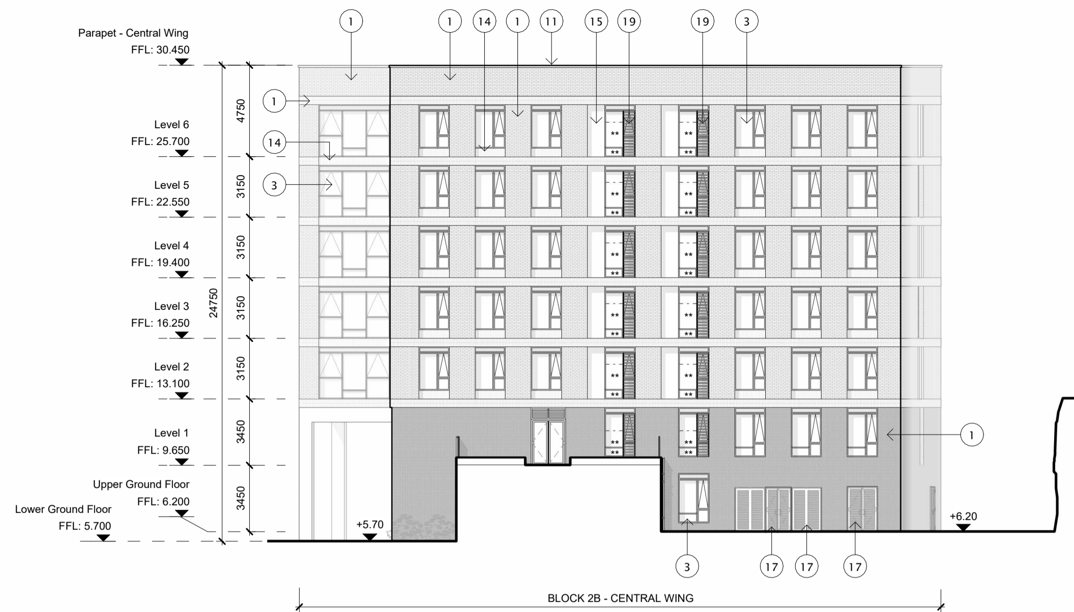
1 Block 2B - Central Wing - East Elevation 1 : 200
