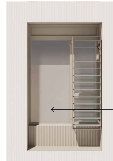
B Type B: Fixed horizontal louvred screen at side panel, with Permanently obscured translucent glazing to fixed panel to 1.8m above FFL
