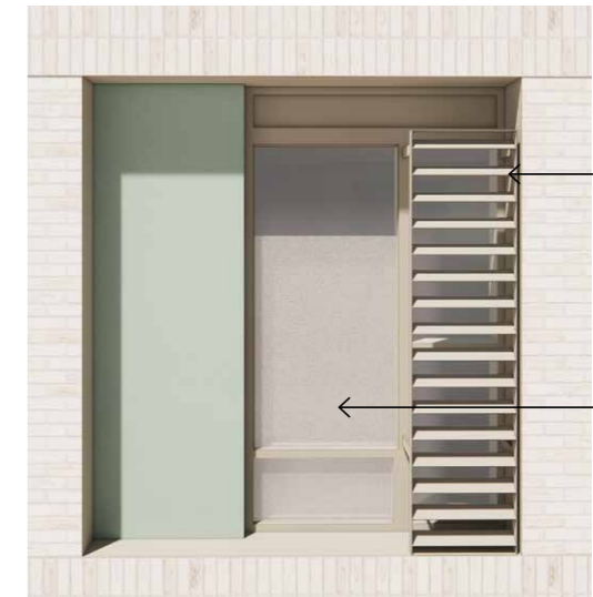
A1 Type A1: Fixed angled louvred screen at side panel, with translucent glass to fixed panel to 1.8m above FFL
