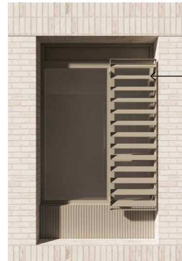
A Type A: Fixed angled louvred screen at side panel
