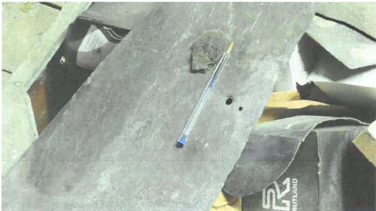
Photograph 004. The photograph shows the oversized (worn) nail hole in the natural stone slate.
