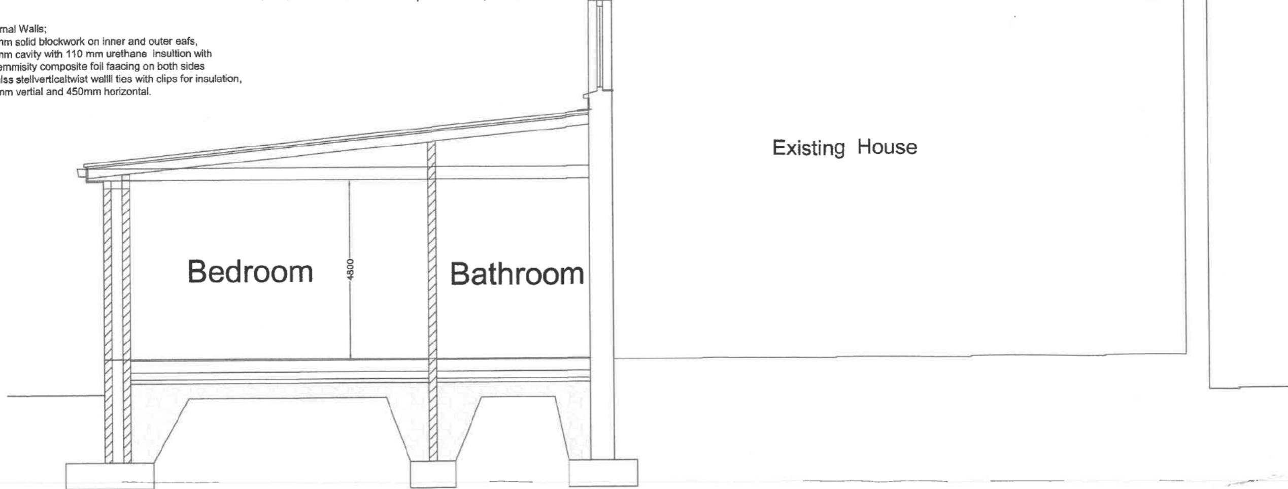
Floor; selected floor finish, on 150mm concrete slab,
