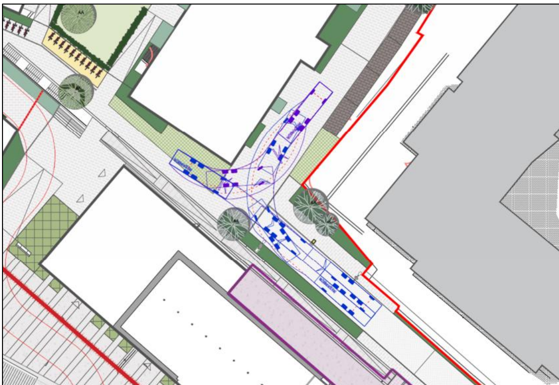
Figure 18.39 Vehicle tracking for waste collection vehicles at Stonetown Terrace (5)
