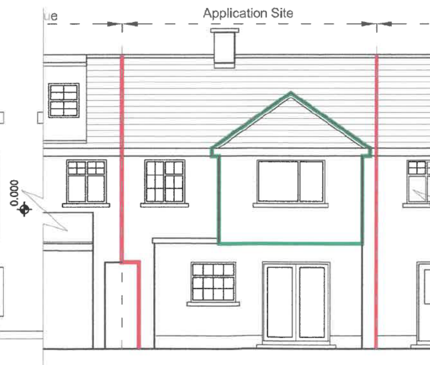
03 West Elevation, Proposed 1 : 100
