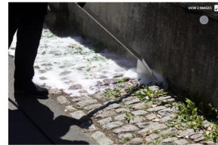
Pictured here being used to kill weeds between cobblestones, Foamstream has recently been trialed on olive groves in Greece. Woodgates
