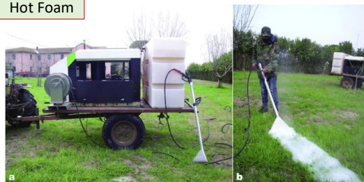
Hot foam machine: (a) lateral view of the machine with the 1000 L water container, the 300 mm wide manual foam hot foam distribution tool, and the covered part containing the foam container, the boiler, the programmable logic controller, the pump and the diesel generator set, (b) hot foam distribution tool and example of a hot foam layer.
