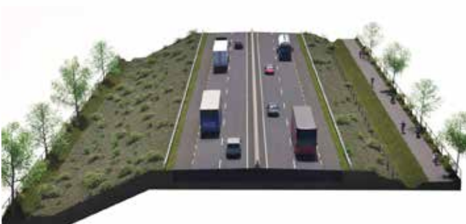
Graphic - proposed N/M20 mainline cross section with active travel.
