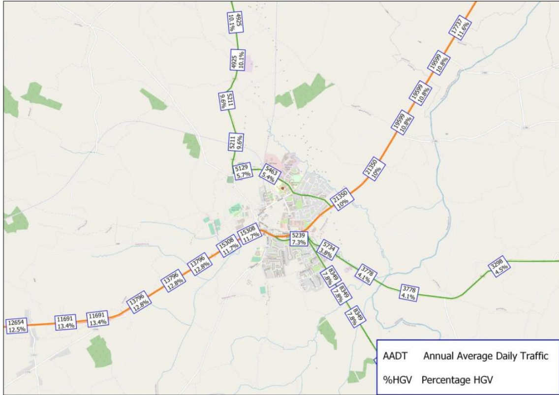
Figure 3.37: The N21 Newcastle West Road Scheme - 2042 modelled future AADT and percentage HGV – Do Minimum (C: Jacobs)
