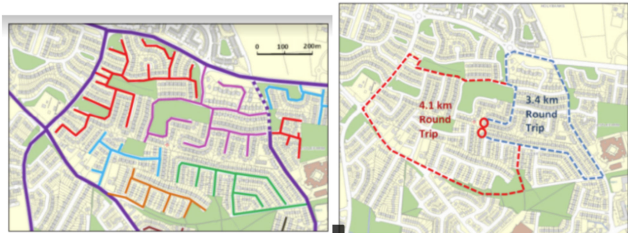
Figure 4.1 DMURS- Typical dendritic spatial layout, restricted permeability
