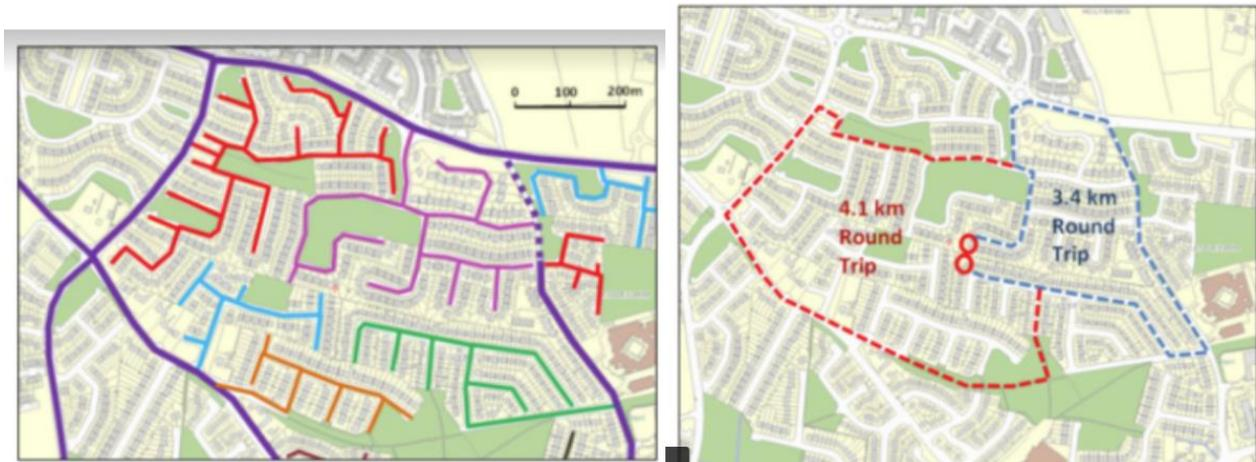
**Figure 4.1 DMURS- Typical dendritic spatial layout, restricted permeability**
