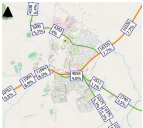
Figure 3.31: The N21 Newcastle West Road Scheme: 2019 modelled AADT and percentage HGV-(C: Jacobs)
