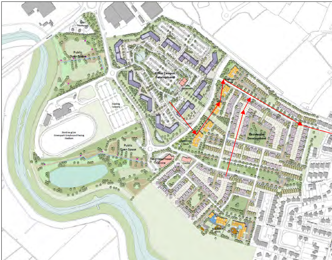
Figure 5.10 Emergency Access and Egress Routes
