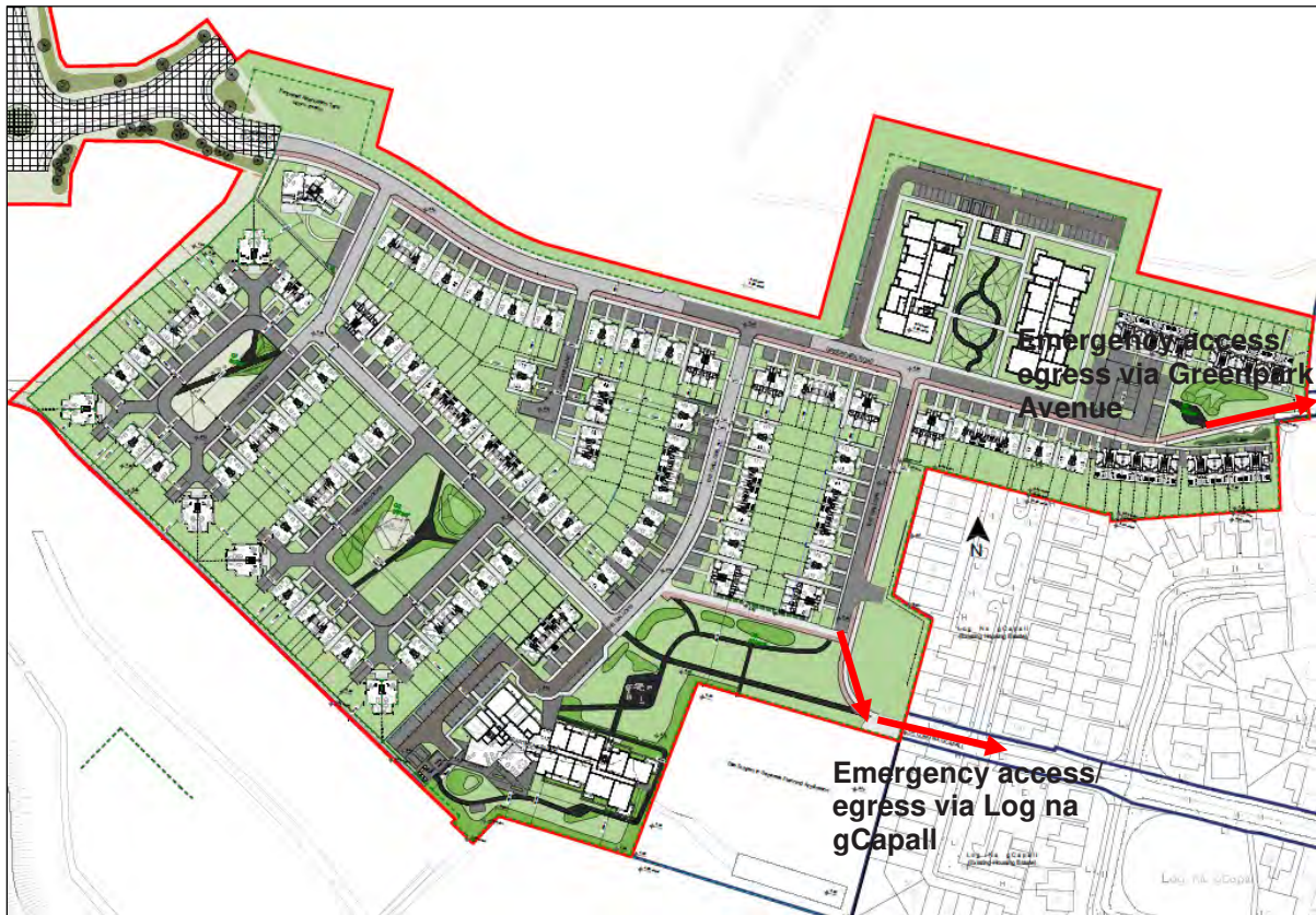
Figure 5.7 Emergency access and egress routes
