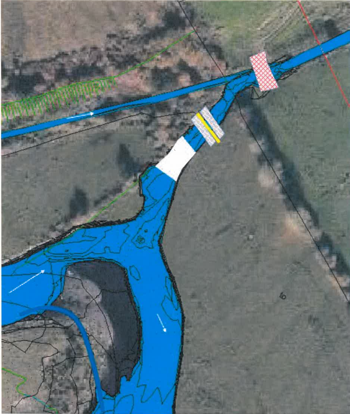
Figure 3.14 STEP 9 Remove all construction equipment and materials from the south and cross the catchment drain. Remove temporary ford construction; Remove the sand bags upstream of the ford; Remove all construction materials from site and reinstate the access road; Remove all construction equipment from site.
