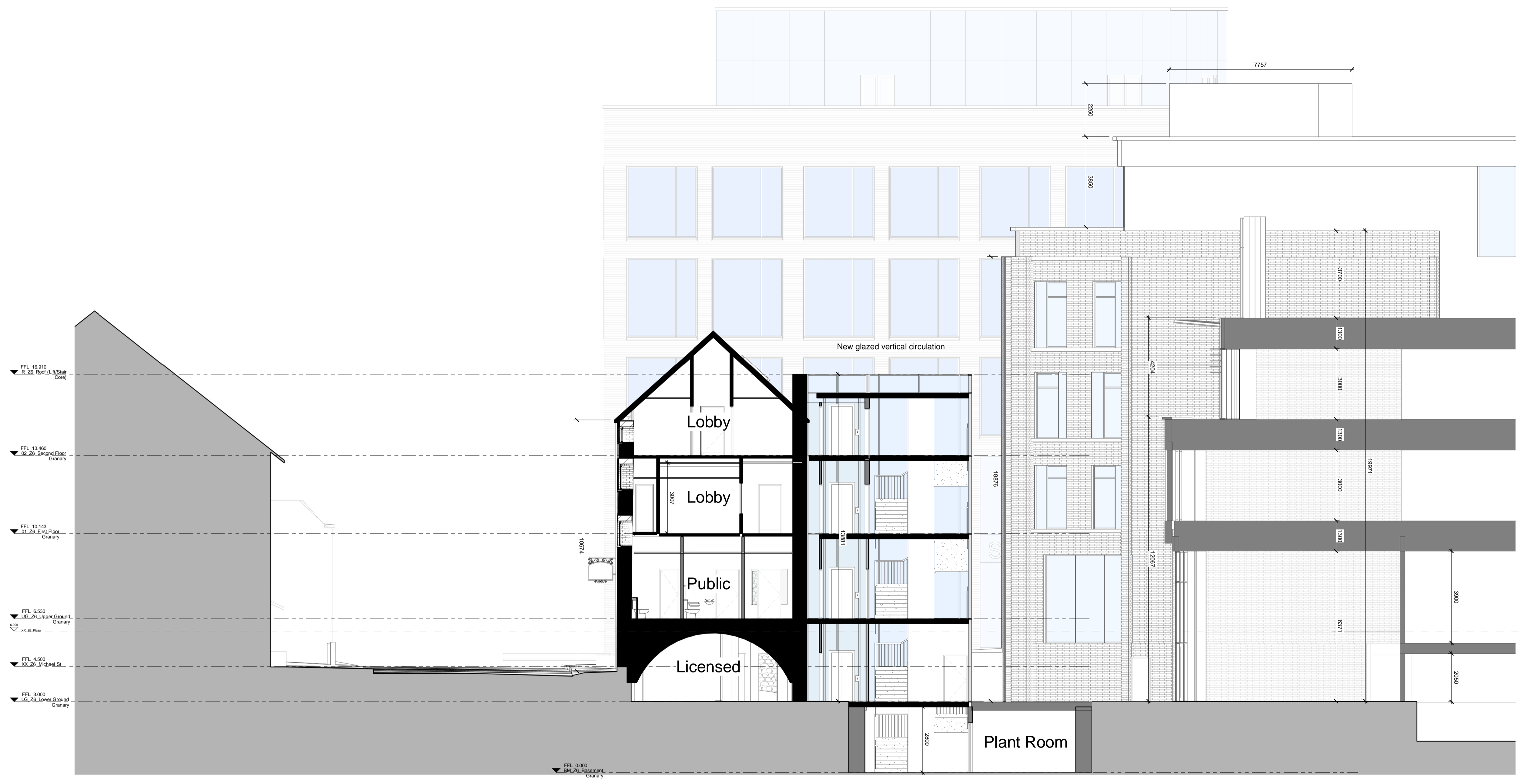
1 Section 1 - Through New Stair Core (South) SCALE: 1 : 100
