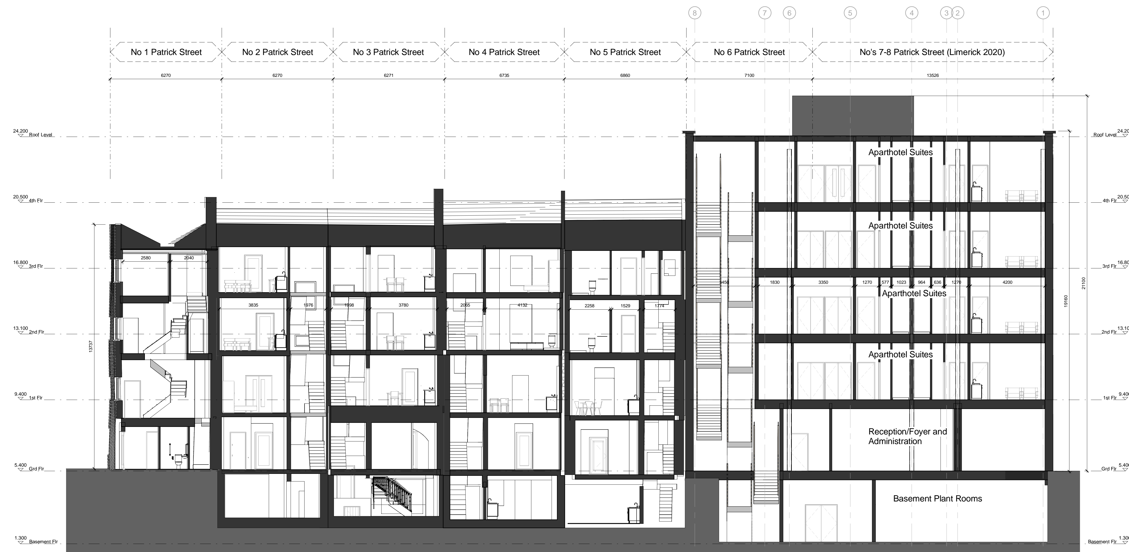
F-F Section through Patrick Street - Proposed SCALE: 1 : 100
