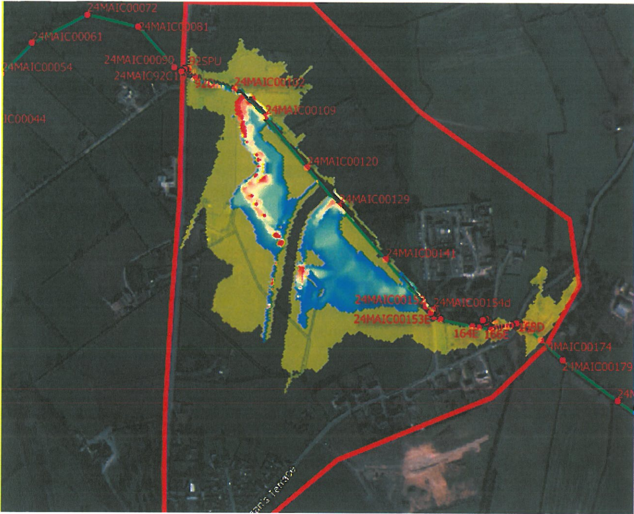
Figure 2: Flood Extent using CFRAM Flows vs Flood extent using Maigue Scheme derived flows (Croom 1d/2d model – Q100 flow)
